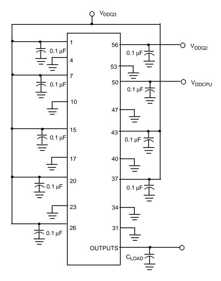
Note: All Capacitors must be placed as close to the pins as is physically possible
